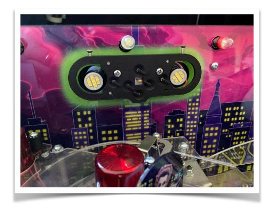
Now simply slide the Sky Cloud onto the backing bracket and insert the screws down into the top of the backing bracket. The screws simply lock into holes on the resin cloud and are not cutting a thread into the cloud reducing the risk of damage / cracking. The thread is pre-cut in the backing mount
