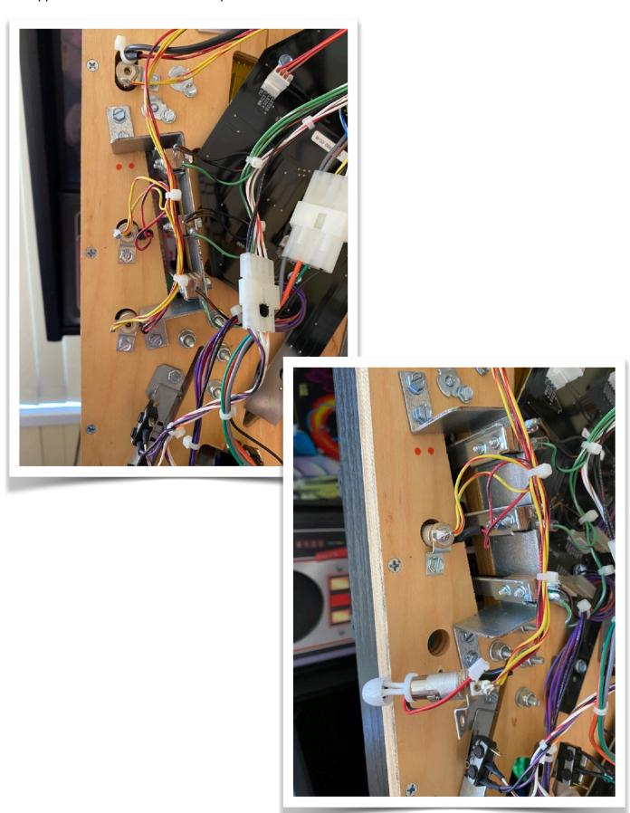
Then re-install the games GI bulb socket back into the playfield but with the adaptor lead sticking out under the playfield.
