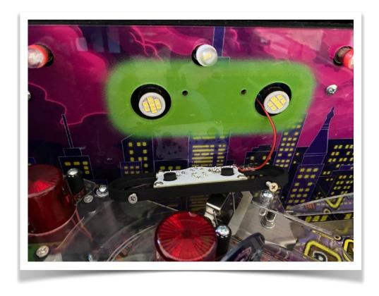
Install the black sky mod plate to the back board using the same 2 screws that fastened the ghost trap to the backboard. The Pro has alot more room where as on the Premium / LE the sky mod is just a couple of millimetres above the top ramp - but the process is the same.
