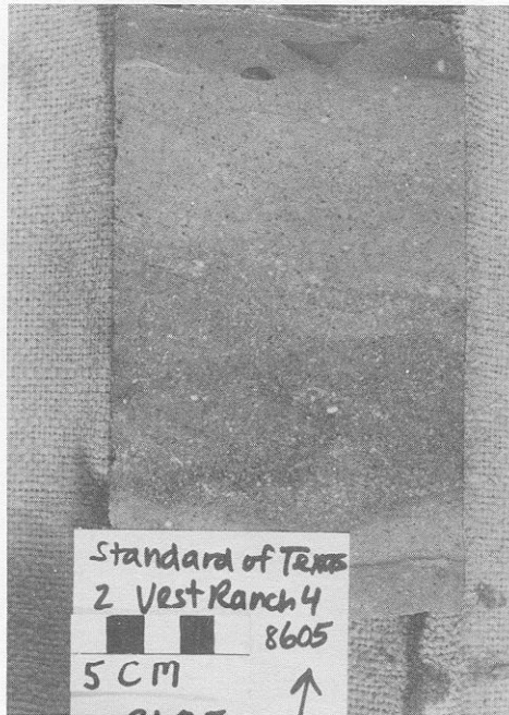
Figure 12. Standard to Texas #2 Vest Ranch "4", Section 4, Block B-13, PSL Survey, depth 8605'. Coarse pebbly quartz sand, moderately well sorted, some cross bedding. This interval comprises part of the pay zone in this well, which has produced (lease average) over 600 MBO/well. This coarse sandstone is interpreted to be braided stream or distal alluvial fan facies. Core depths were suspect in this well due to poor depth marking and core preservation.
