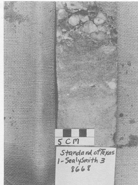
Figure 19. Standard of Texas #1 Sealy Smith "3", Section 8, Block A, G&MMB&A Survey, depth 8668'. Sandy, well sorted, crinoid wackestone/packstone, immediately overlain by a coarse chert pebble grain-supported conglomerate. Periods of shallow marine deposition were interrupted by coarse debris flows.
