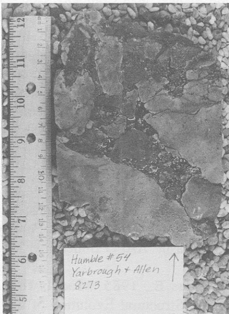
Figure 18. Humble #54 Yarbrough & Allen, Section 9, Block B-13, PSL Survey, depth 8273'. Cobbles of algal limestone, weathered red, in a red shale matrix. This was a shallow marine limestone capping the chert conglomerate facies, which was subaerially exposed and weathered; a terra rossa surface.
