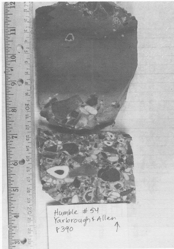
Figure 22. Humble #54 Yarbrough & Allen, Section 9, Block B-13, PSL Survey, depth 8390'. Chert cobble conglomerate, ungraded, clast supported, chert pebbles have deeply weathered rims. This conglomerate has a siliceous matrix, and is capped by a 4" (10 cm) bed of homogeneous chert. These siliceous beds were rare in the cores. They probably represent a diagenetic phenomenon such as the formation of a silcrete horizon during pedogenesis.
