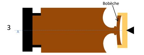
Put a tight fitting cap over the top. If necessary, use tape or a paper towel to get a tight fit. Mark the position of the cap on the wood. Using the tailstock for support, cut under the Bobèche. Sand smooth.
