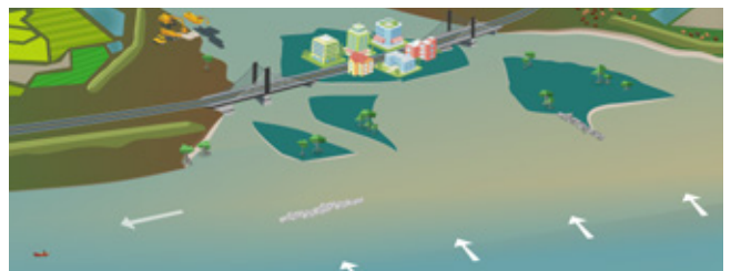
Fig 6b: The coast scale after human intervention. Coastal replenishment of sediments from rivers and sea currents is reduced. Sand transported by longshore currents is trapped behind groins and seaports. Beaches, sand bars and sand dunes erode.
