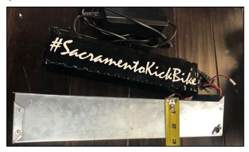
One crossmember had to be cut out from under the deck to fit the battery, there were wiring, connectors and some soldering for it to all function properly. If you are good at wiring and soldering this will be a breeze. If not, hopefully someone will put together a kit that is plug and play soon for these kick bikes. Or if they are still available you can purchase an E-Cruiser Deluxe already assembled @ <a href="https://sacramentokickbike.com">https://sacramentokickbike.com</a>
