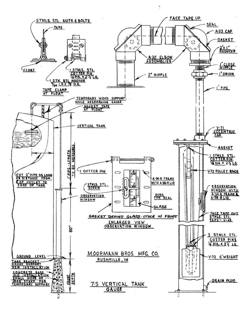
START TAPE, CLIP END FIRST WITH NUMBERS ON TAPE FACING FRONT OF GAUGE HOUSING, AROUND LARGE BOTTOM PULLEY, UP TO LARGE TOP PULLEY, DOWN TO MEDIUM BOTTOM PULLEY, UP TO MEDIUM TOP PULLEY, DOWN TO SMALL BOTTOM PULLEY, UP TO SMALL TOP PULLEY AND THEN SECURE CLIP END OF TAPE WITH A COTTER PIN TO THE TOP OF THE BOTTOM PULLEY RACK (V-73) ASSEMBLY.
