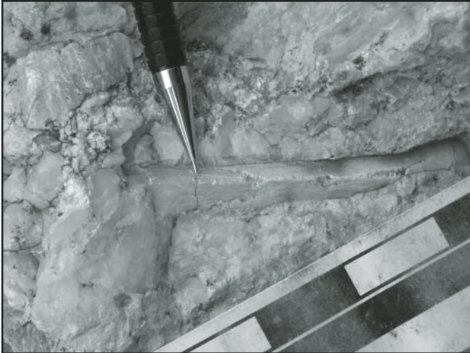
Figure 9. Constant volume replacement of quartz. Light green talc has completely replaced the original euhedral quartz crystal extending right to left across the center of the photo at the pencil point and other quartz grains in the left and upper portions of the photo. In this pegmatite, the talc is a pseudomorphic form after quartz, but feldspar remains relatively fresh even where it is immediately adjacent to quartz that is replaced by talc. Fresh quartz is present in this sample just to the left of the pencil point and exemplifies an abrupt alteration boundary. Pegmatite from the Granite Creek area in the southern Tobacco Root Mountains. Scale is in inches.
