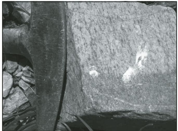
Figure 8. Loose block of pink quartzofeldspathic gneiss (i.e., Dillon Granite Gneiss) from the Treasure Mine area. Biotite in the gneiss in the upper part of the photo is partially replaced by chlorite but the feldspar and quartz are unaltered. The gneiss below the sharp boundary extending horizontally across the lower part of the block is strongly altered to chlorite and contains quartz veinlets. Individual foliation surfaces can be followed uninterrupted across the alteration boundary. Bird droppings (white elongated blot) are oblique to boundary. Rock hammer provides scale.
