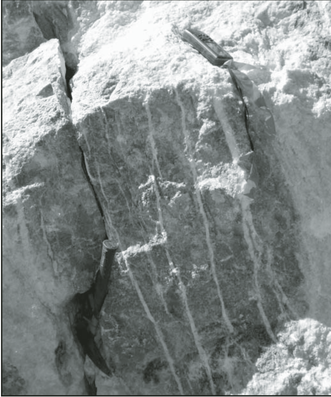
Figure 3. A loose block of ore in the Treasure Mine showing some of the complex relationships between talc and carbonates. The central domain of medium-green chloritic talc is cut by white veinlets <1 cm thick of dolomite or magnesite. These veins terminate at the contact between the chloritic talc and the surrounding coarsely recrystallized white dolomite. The recrystallized dolomite is partially replaced by white coarsely crystalline talc. Hammer and GPS unit provide scale.
