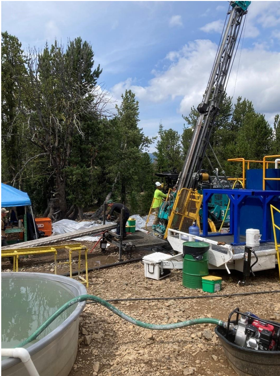
Figure 58. Core drill rig on hole CZ-2021-01 in the CZ deposit on the northwestern ridge of Iron Mountain (Photo: John Childs).
