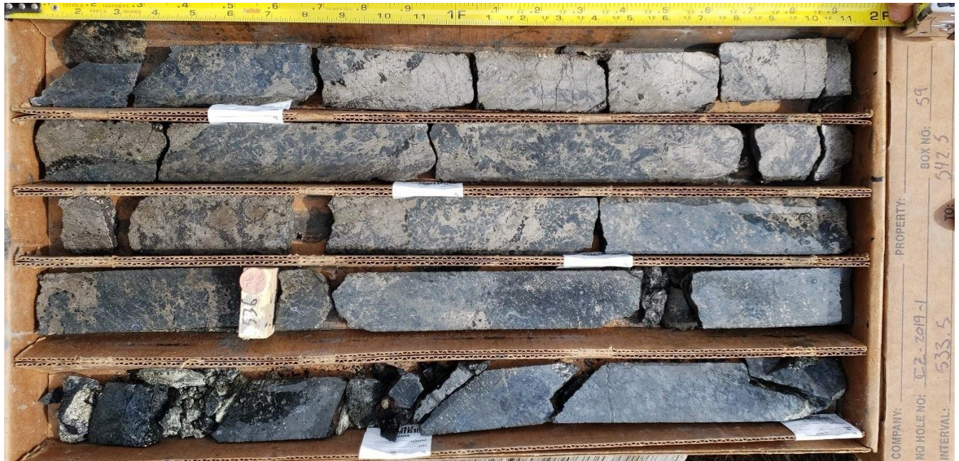
Figure 15. Net-textured to massive sulphide interval at 533 to 542 feet in core hole CZ-2019-1 (Photo by J. Modroo).
