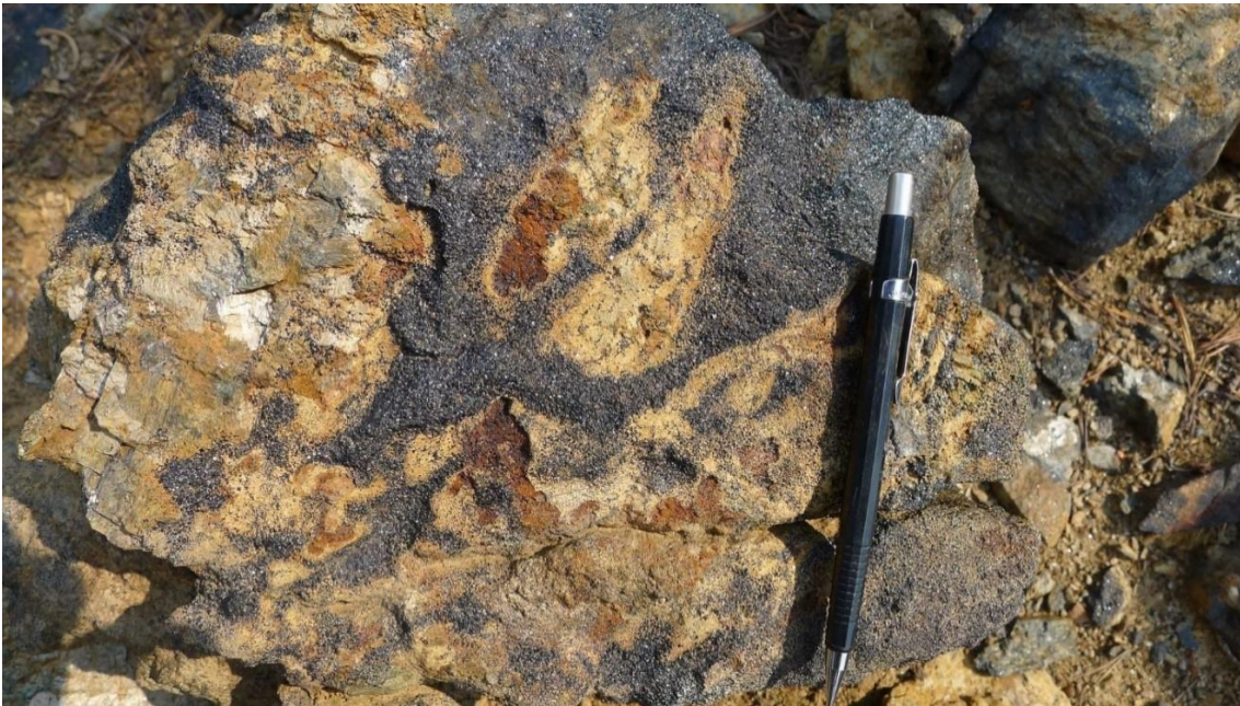
Figure 28. Pegmatoidal Bronzite with lenses of chromite from the Hybrid deposit. A sample from this outcrop carried 4,606 ppb 3E (Photo by C. Bow).
