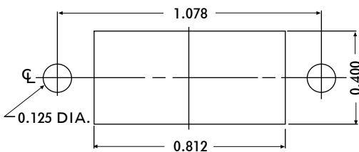
RECOMMENDED CHASSIS CUT-OUT
