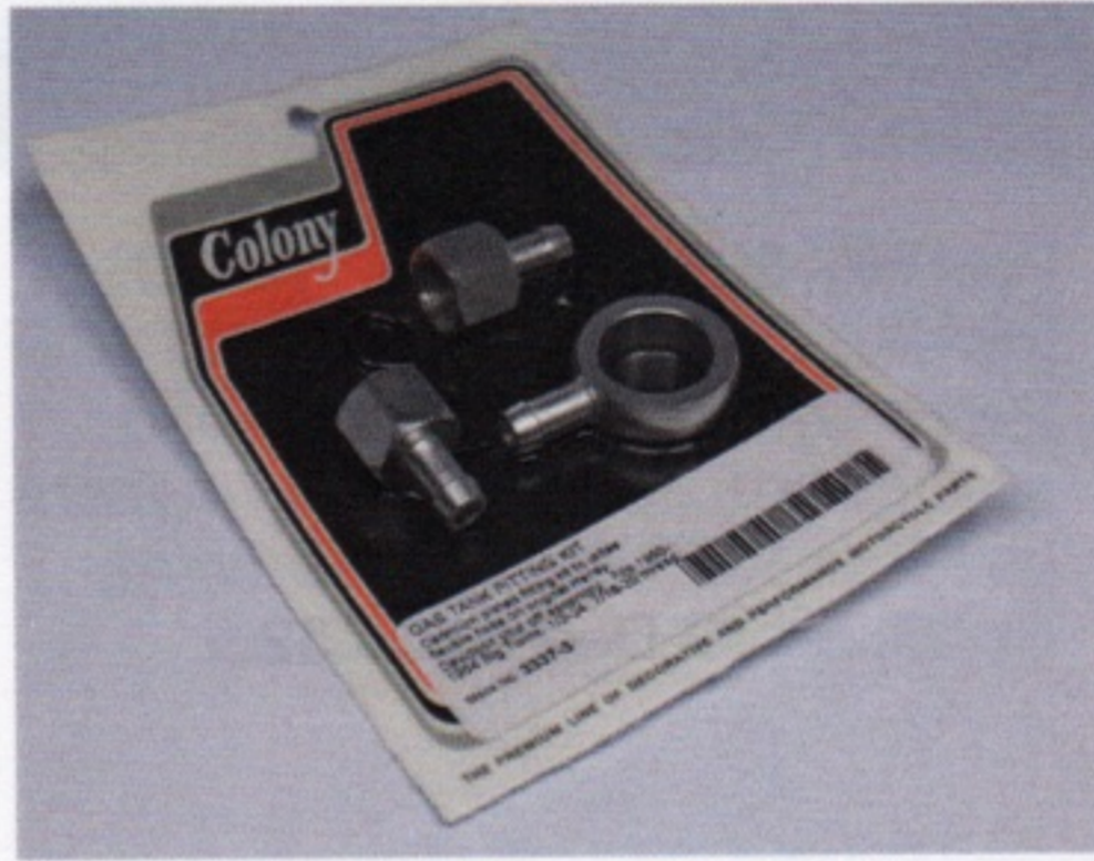
Part No. 3337-3 GAS TANK FITTING KIT Cadmium plated fitting kit to utilize flexible hose on original Harley Davidson shut off assembly. 1964 Big Twins. 1/2-24, 7/16-20 thread. Retail: $19.34
