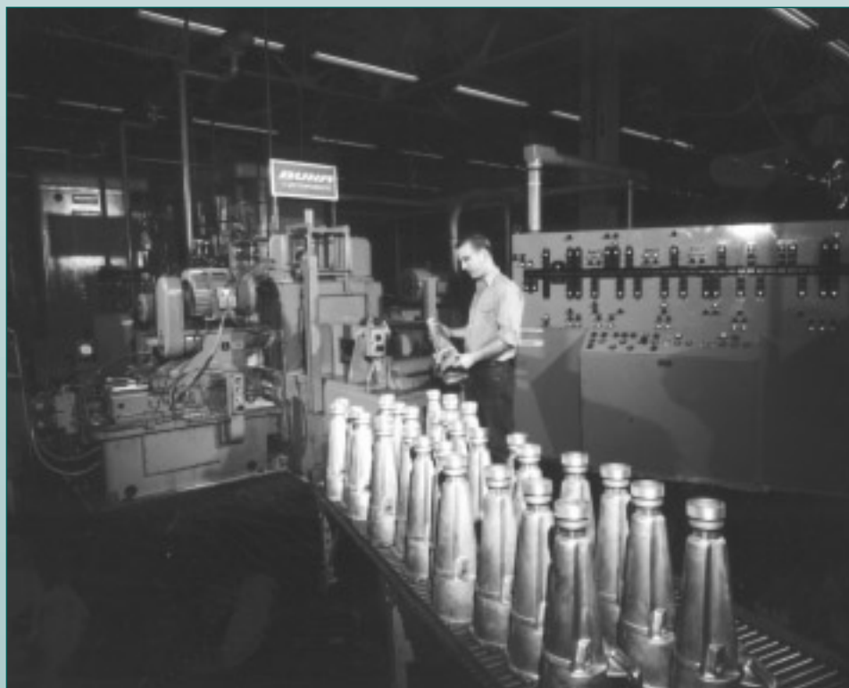
Extension housings being machined, late 1950s
