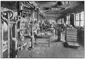
Figure 3: Typical drive shaft plus pulley structure in a factory.<sup>22</sup>
