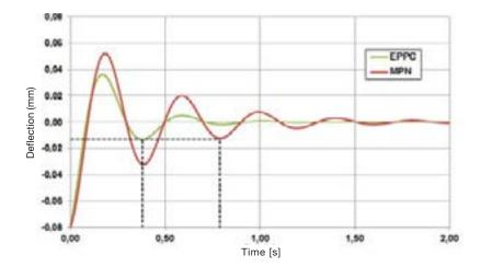
Theoretical MPN vibration curve compared with EPPC™. At a deflection of -80 µm the MPN reaches a stable position within a tolerance of +/-15  $\mu$ m after 0.75 seconds. With EPPC $^{\text{TM}}$  the deflection time is reduced by 45 % to 0.4 seconds
