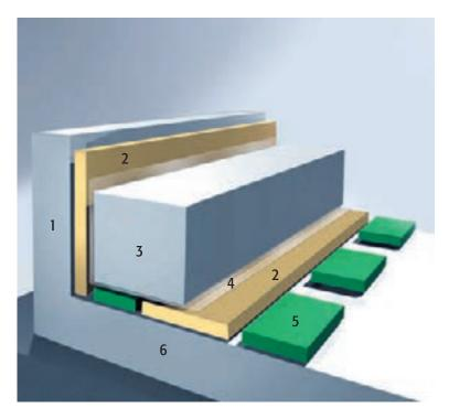
Insulation pads are perfectly suitable for the vibration insulation of foundations
