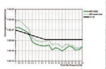
Result of vibration measurements on a foundation block insulated with Bilz membrane air springs.
