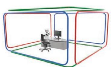
Bilz magnetic field compensation using room coils
