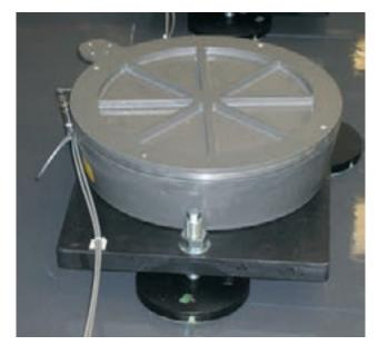
The foundation insulation using low-frequency BiAir® membrane air springs enables an optimum insulation effect. Unlike with the use of pad sets or steel springs the adjustable level of the foundation block automatically resets itself in response to load changes through the level control.
