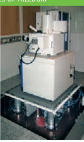
Application example: Electron microscope on a vibration insulating platform
