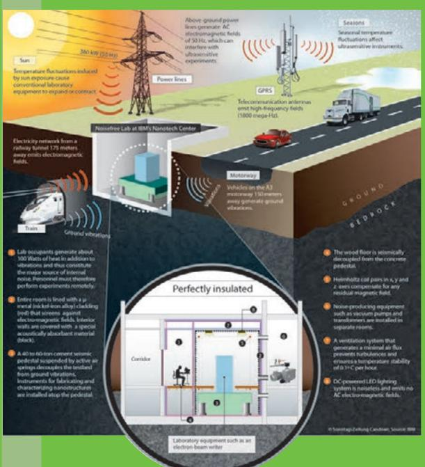
The illustration shows some of the most important measures for reducing external disturbing influences in the "noise-free labs" of Binnig and Rohrer Nanotechnology Centers of IBM and ETH in Zurich.
