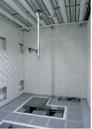
Experimentation room with 4.2 m clear room height and acoustic insulation materials (supplied and installed by Bilz).
