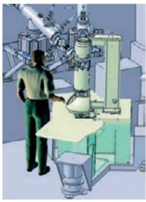
Electron microscope on a vibration insulating platform
