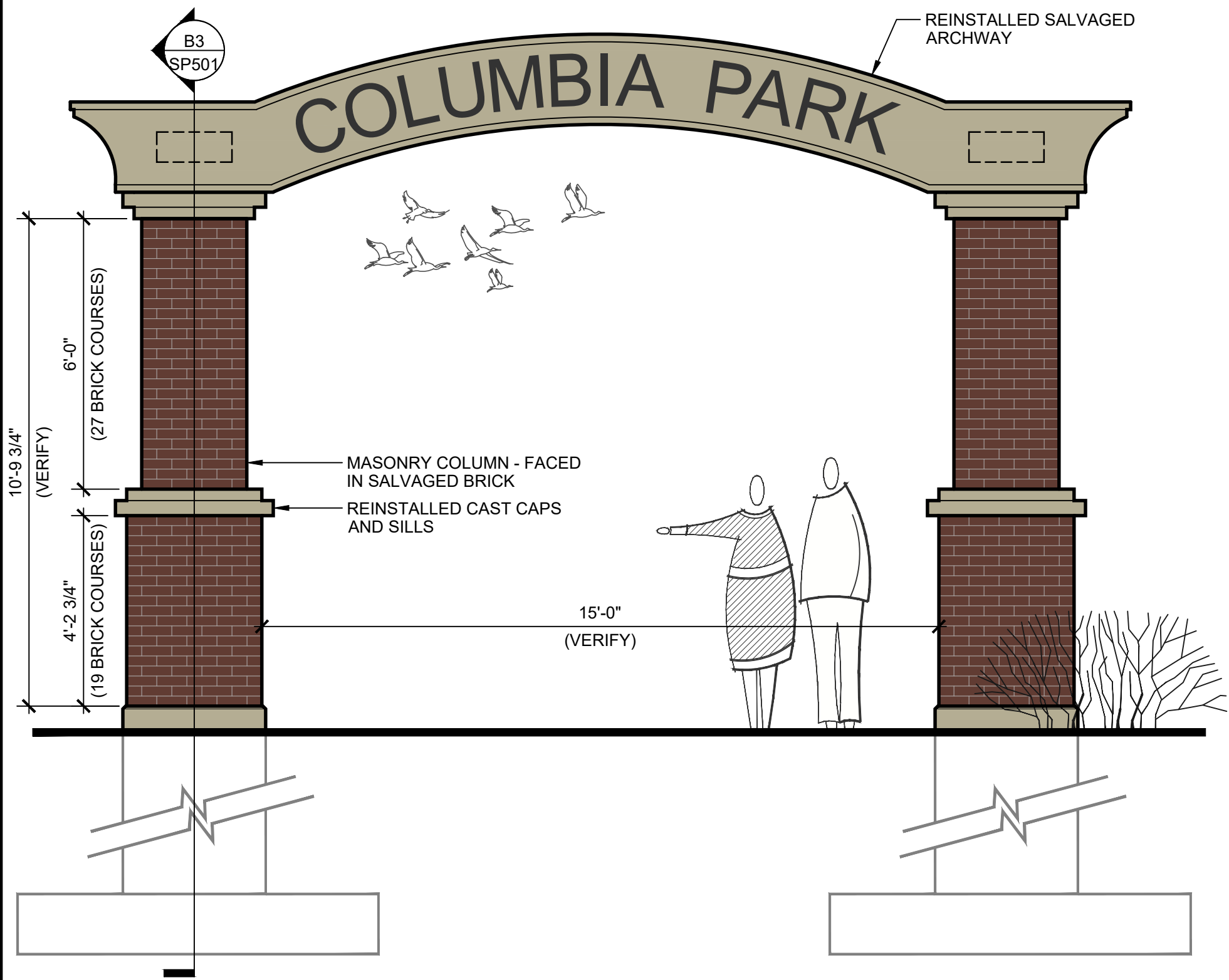
B1 SP501 ELEVATION: RE-CONSTRUCTED HISTORIC ARCHWAY SCALE: 3/8" = 1'-0"
