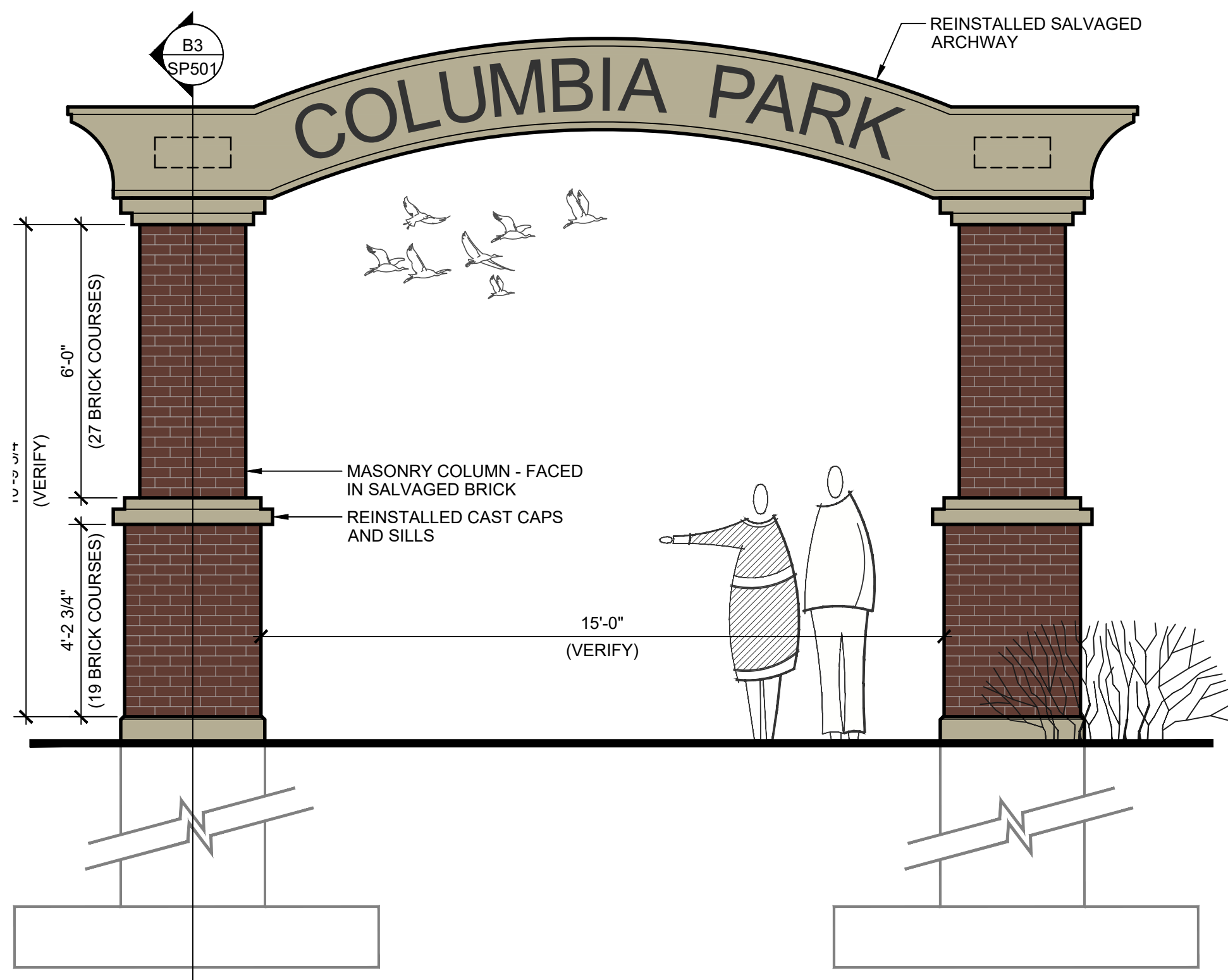
B1 SP501 ELEVATION: RE-CONSTRUCTED HISTORIC ARCHWAY SCALE: 3/8" = 1'-0"
