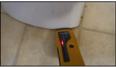
Basement toilet may be leaking at wax seal
