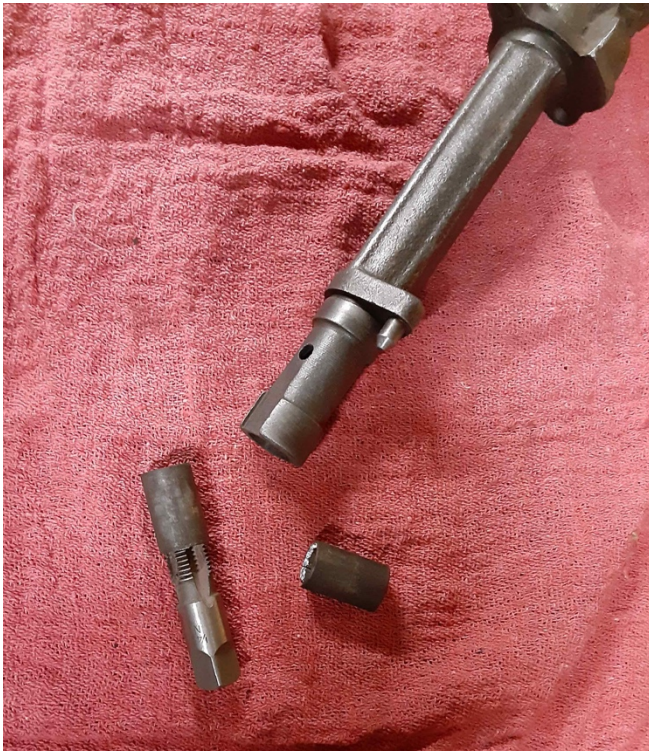
Photo five: Here is another trick to use an old shaft from the oil pump / distributor drive as a mandrel to press in the new bushings.
