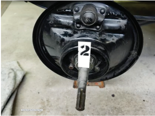
One of the front spindles and backing plates ready for new brake shoes.
