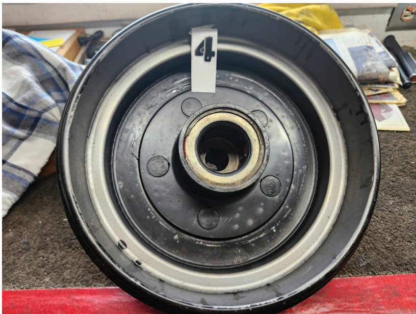
New brake drum with new grease seal and snap ring installed, ready to be put on the spindle.
