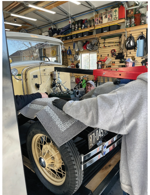
Back on top, Bill watches anxiously as the old motor is lifted out of the frame.
