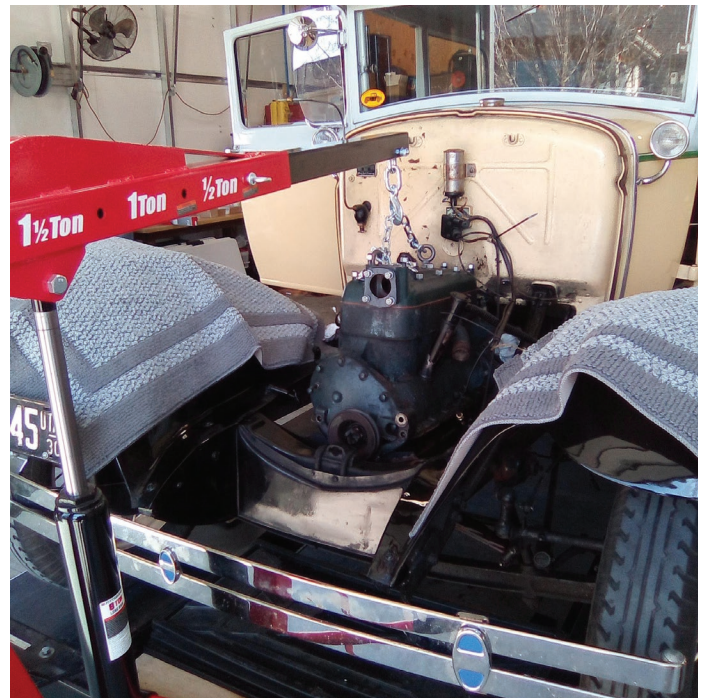
The "cherry picker" hooked up to the old engine, ready to be removed.
