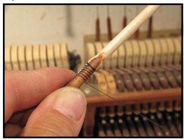
One example of a part which might need to be replaced or repaired on a grand piano would be that of a broken hammer shank. Each shank connects to a hammer, and as such is subject to a great deal of stress and occasional breakage. In the photo left, a new section of shank is spliced to the bottom of an old shank which had broken.
