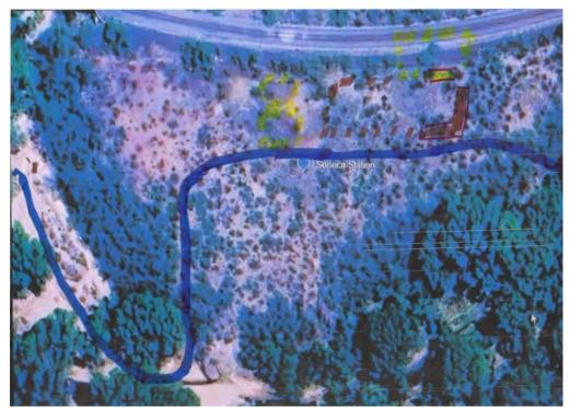
Seneca Station: Blue line is the road. The cuts make this almost certain. Solid yellow line surrounded by red line is the remaining foundation of an adobe wall. Dashed yellow is a guess at what might have been. Discoloration of the ground cover may indicate the former locations of structures. Loose stone outlines these spots. Brown line surrounded by red is the foundation of a stone wall. Dashed brown line shows the probable location of the rest of this wall.
