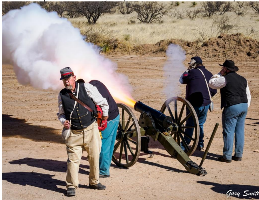
The 12-lb Mountain Howitzer which could be disassembled and packed on mules was widely used in the Indian Wars
