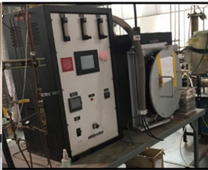
F) Retort-Lined Furnace for Inert, Oxidizing, or Reducing Atmosphere Control to 1100 °C
