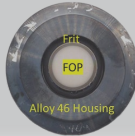
Thermal Expansion Matched Glass Frits used for Sealing Assemblies for Alpha Detection
