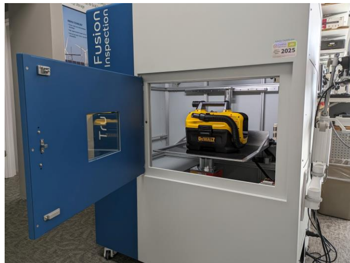
20"x20"x20" stage and chamber accommodates large parts (vacuum)
