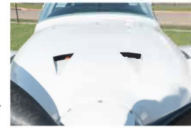
Air Cooling Inlet
