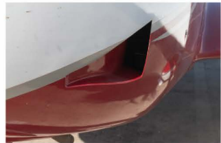
Induction Air Inlet
