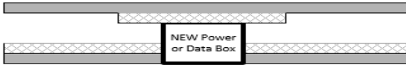
Option 1: worker to install new power utility wall box and add Lead Lining to wall behind box If worker can access posterior wall entry
