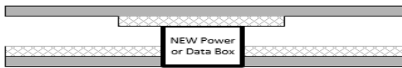
Option 1: worker to install new power utility wall box and add Lead Lining to wall behind box If worker can access posterior wall entry
