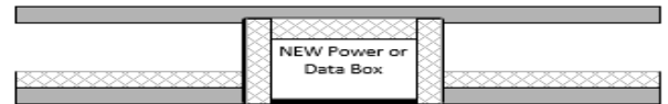
Option 2: worker to install new power utility wall box – box is lead Lined by manufacturer
