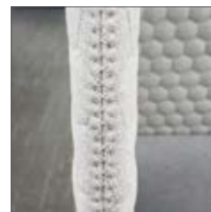
Cross-stitching (Panel seam)
