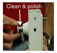
machine oil such as 3-IN-1 oil, then reinstall crank socket and E-clip.
