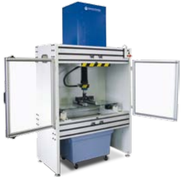
Special purpose machine for determining the breaking strength of glass
