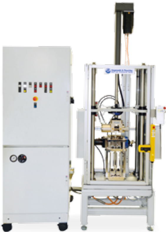
Special purpose machine for the draw bead test on body sheets
