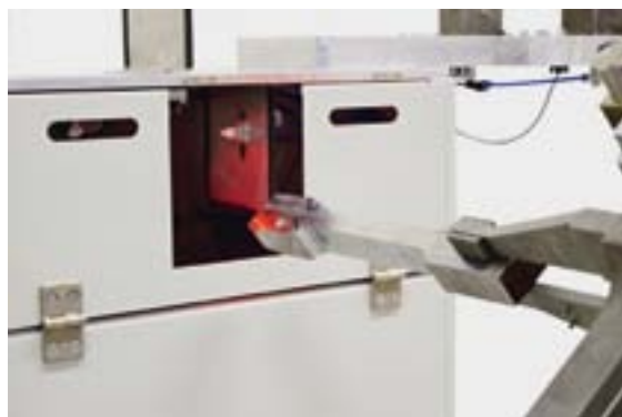
Optical measurement of the specimen in the automated test centre
