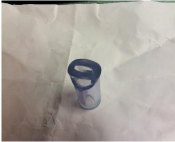
Sight gauge tubing material after being crushed flat in a vise. No cracks or breaks.
