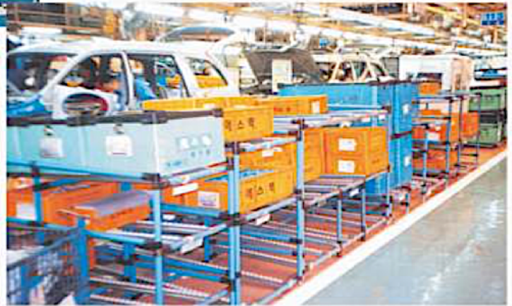
MAIN ASSEMBLY LINE RACK FOR AUTOMOBILE
