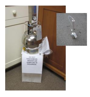
Laboratory supplied stainless steel Summa canisters are utilized to collect air/soil gas for the required analysis
