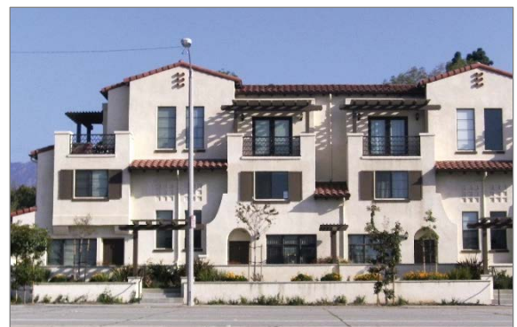
A modulated façade and varied rooflines prevent a large residential project from appearing overwhelming and out of scale.
