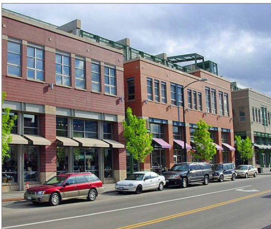
A parking structure “wrapped” by commercial and residential space conceals the parking and allows for windows and active uses to face the street.
