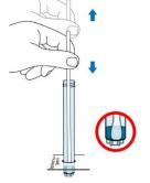
7. Make sure the swab tip is in the liquid inside of the tube. While using one hand to securely hold the tube down, use the other hand to carefully break the swab handle against the side of the tube. Discard the swab handle and leave the broken swab tip in the tube.
