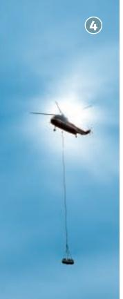
**4** Self-reliant jobsite. SBBI flies cement into the site and removes aggregate directly from the river. They feed both materials into their onsite portable concrete plant for fish-barrier materials.
