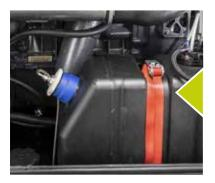
**DEF TANK** The approximate consumption of DEF tank is about 10% of the diesel oil consumption. The DEF tank is heated to prevent the urea from freezing.
