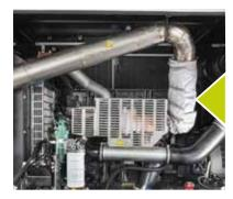
**EXHAUST GAS** Exhaust gas comes out of the engine as yet untreated but already with reduced emission levels thanks to an efficient electronically controlled engine and a common rail injection
