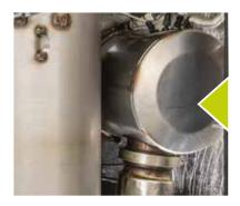
DOC | DIESEL OXIDATION CATALYTIC
