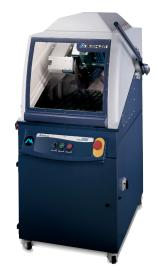
Allow for sectioning of parts with a 3.5in [88cm] diameter. (Varies based on part shape)
