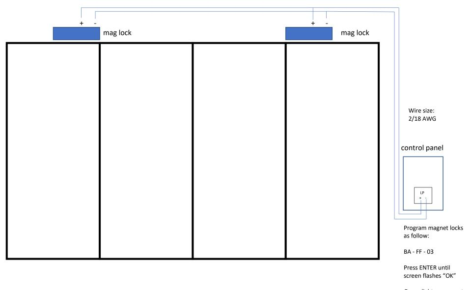
Green light on magnet no contact Red light on magnet good contact
