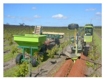
TG Drains can use different methods for delivering gravel into the machine's hopper depending on where the drainage is installed. For vineyards we use a gravel trailer with an elevator belt to bring the gravel up and over the rows of vines.
