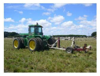
Mole channels must have an even, gentle grade, with minimal grade changes. TG Drains uses a floating beam mole plough to install the mole drains. A floating beam mole plough allows the expander to maintain itself at the set depth irrespectively of small ground surface irregularities and allows the ripperleg and the expander to produce a smooth gradient to the mole channels.
