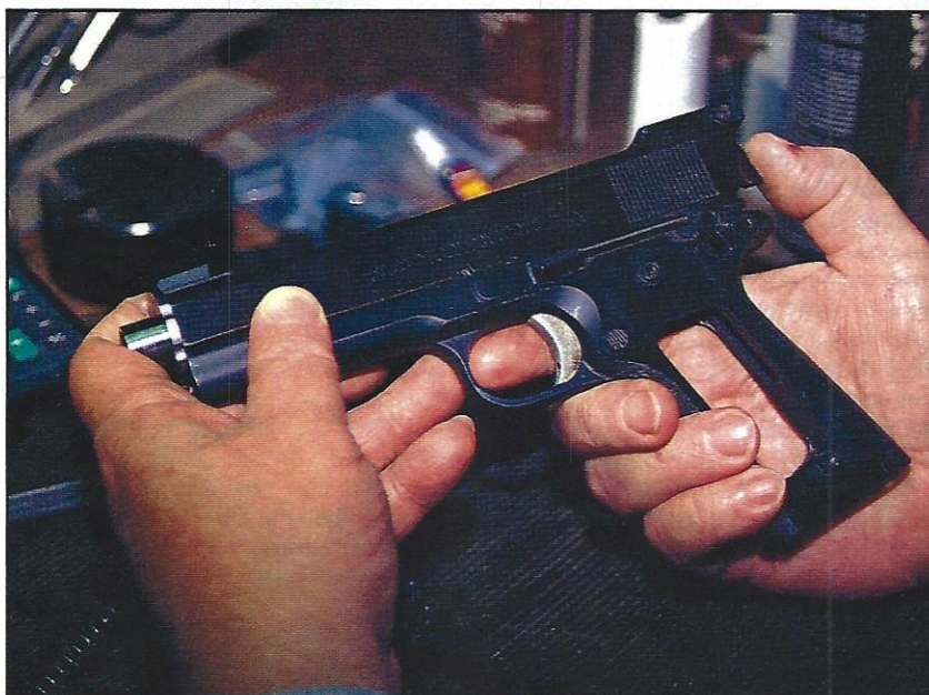
You can feel the slide begin to go into battery as the fitting progresses.
