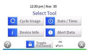
The Cycle Use Information History screen can be reached by selecting the "Cycle Usage" button. It will display the past cycles run on the unit which may be scrolled through using the arrows on the right of the screen. Additionally, there will be a "Back" button to return you to the Select Tool screen and a "Delete?" button. The "Delete?" button will prompt an alert to confirm the previous cycle's information is deleted.
