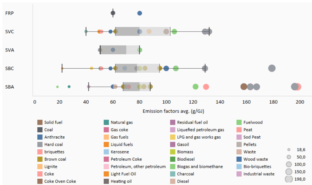
Figure 17. NOx emission factors for each type of fuel and technology in the EU27 residential subsector, 2020, as reported by sixteen MS (g/GJ)
