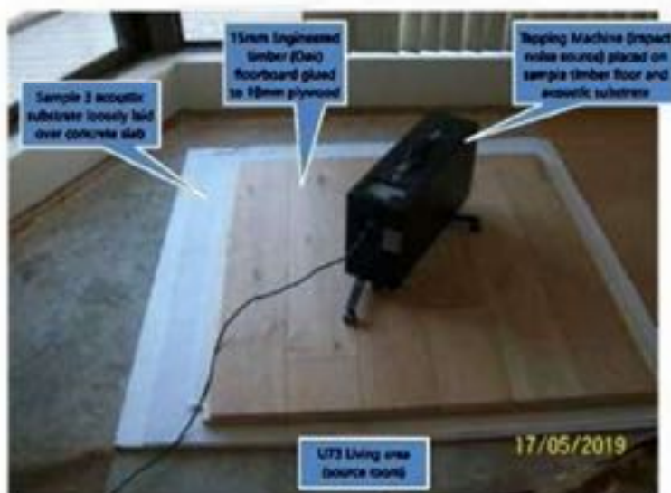
Figure 1: Typical Sample Floor Setup Test In Source Room (Unit 73)
