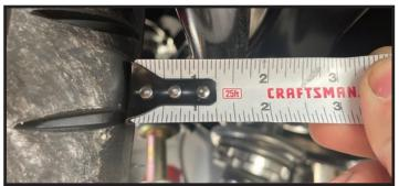
With ¾' at play, it clears more than enough for this application. The sway bar moves on the same plane as the control arms, so no worry of changing clearances here. We know from our hub-to-fender measurement and this measurement we'd have \*some\* amount of room to go wider overall....but this is really pushing it.
