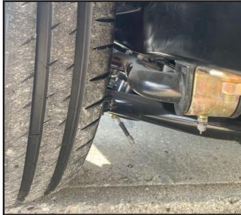
With the wheel and tire bolted up, we find what is undoubtedly the tightest point of the system: the front sway bar. Too much backspace, and the front wheel rubs at full lock. No sway bar? Not as big of a problem, but being as this is one of the most common modifications, and those big modern hoops would be a waste without one, this is going to be commonplace for most. This measurement being as tight as it is, is partially
