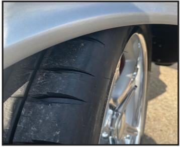
coilover suspension packages. And shown here, is spun almost all the way down on the adjusters. So, a quick couple turns up of the collars, and a happy medium is found.
