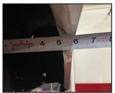
Now, onto the measurements! First, we go from the face of the brake rotor, to the fender lip. Take your favorite straight-edge, place it on the rotor where the wheel would set against, and measure out. We see here we maintain a distance of 5". With our 7" wheel having 4" backspace, and .75" of bulge, 3.75" total from the face of wheel lets us know we more than pass the finger-width test..... at least while going straight!
