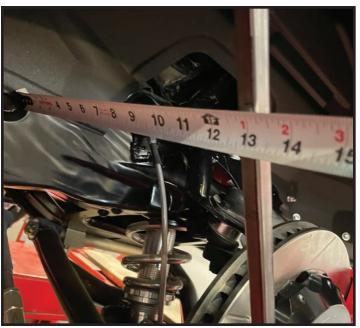
Rear inner fender clearance measurement is a little more difficult to do. You'll be looking for the tightest point, which will wind up being the back curve of the inner fender. This measurement of 12.75" means basically whatever we stick in here will work....until we start turning.....
