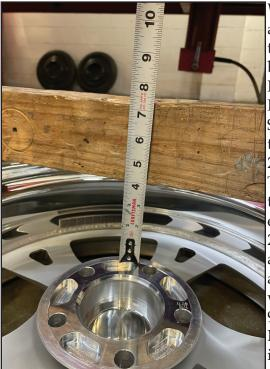
Wrapped around these beauties are Michelin Pilot Cup Sport tires, in 235/45zr18. These are rue to equate to 26.3" tall, and have an overall width of 9.25" static. Now, installed on a 7"
