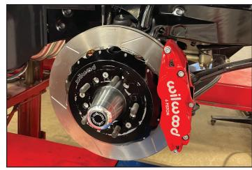
but maintain factory track width. The bigger the rotor, the bigger the wheel will be required. Again, your brake manufacturer will be able to provide these specifications.
