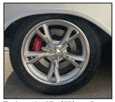
The aforementioned "low." With our coilovers turned up far enough to simply close up any gap between the fender and tire while pointed straight, instead of "tucking" the top of the tire, this setup will have plenty of clearance at lock, even on an uneven surface.
