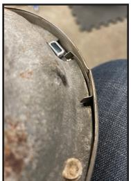
On the backing tray, there'll be three notches to orient the headlight itself, which only go one way. There's also a notch to orient the trim ring, positioning the adjuster tabs in the correct location and keeping all your lines perfectly vertical. Once everything is assembled, plug the
