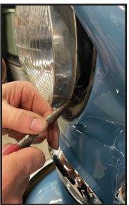
With the bezel removed, the next step is to remove the retention spring on the right side. A pair of needle-nose pliers are my weapon of choice here, there's not much room for anything else, and a clamping tool of sorts allows you to keep control of the spring.
