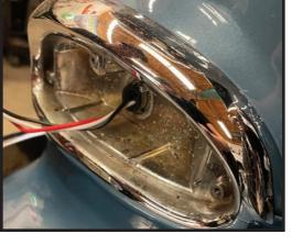
remember to put the original lens-to-housing gasket on the LED lens first!
