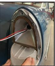
Just as the park lights, the tails use an 1157-style socket. If your car is equipped with back up lights, you can add LED flavor to those at this time as well by tagging on P/N 14542. Our unit here is not so equipped.
