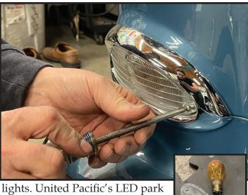
lights. United Pacific's LED park lights replace the lens, so no need to remove or modify the actual housing in any way shape or form.
