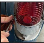
With the bezel out of the way, the retention 'bar" for the backup lights and taillight is removed.
