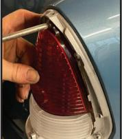
Loosely fit the stainless bar into place. Once all the recesses are lined up properly, cinch this down along with your upper screw.
