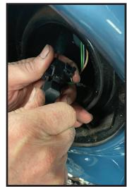
3-prong plug into your factory wiring. Again, there is no modification needed here. I always recommend a dab or dialectric grease in the connector to inhibit corrosion. Carefully feed the wire into the headlight bucket, and slip the tabs on the stainless ring into the adjusters.
