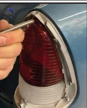
With the bar removed, the upper screw holding the taillight lens is taken out and the lens and bulb are discarded as neither is used over.
