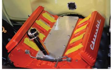
The finished product, ready for trimming. Note the use of masking tape over the intake ports. Don't want anything getting down in there while you're drilling, just remember to take them off before mounting the intake. Ask me how I know....
