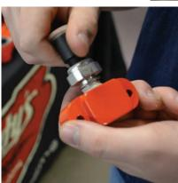
Once screwed together, you can install the adapter on your pan. Depending on your harness, some unwrapping or extending may be required to reach.
