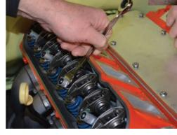
The spacers are studded on the bottom, and install right to the factory bolt holes, in order to utilize a short, taper head
