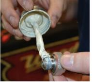
The LS Classic valley pan also relocates the oil pressure sender down to the oil pan, so removal is required.
