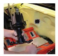
As you can see here, the "shaft" is actually hollow, and oversized so it can accommodate all wires passing through it. The mounting tabs bolt through the two rearward valley pan bolts.
