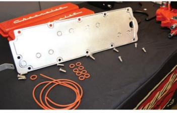
Our new valley pan has CNC machined oil blockoff provisions, as well as the gasket seal.
