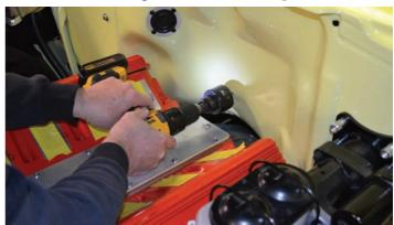
A 2.5" hole saw will be the weapon of choice for cutting the firewall. A uniform hole is key when using the type of grommet we have planned.
