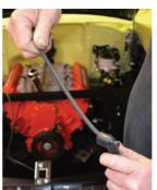
The plug wires come with the sparkplug end of the wire preassembled, so you'll be working from the plug-back. The fake boot is slipped on over the wire, which is sent through the distributor, into the car, where the coil end is crimped on.
