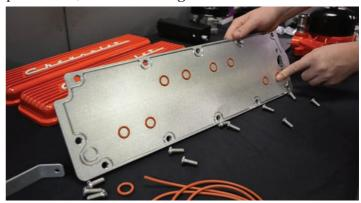
The oil galley blockoff seals should fit snugly in place. The machining on the valley pan truly is impressive.
