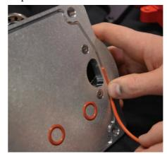
The outer seal will need to be cut to length, but have no fear, it's easily done. Just feed it all into place.
