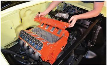
With the intake out of the way, the valley pan is easily removed. No sealant or anything to scrape off, you'll find most all gaskets on the LS series engines are o-ring style.
