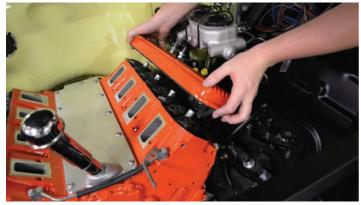
With the spacers in place, including the allimportant o-rings, installation will simply be reversal of removal.
