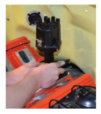
Since our ignition coils are inside the car, we need to put a hole in the firewall for the plug wires to pass through. So, we mock everything up, and mark the firewall directly behind the distributor to keep everything as hidden as possible.
