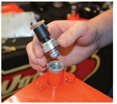
A neat, billet aluminum adapter is provided, and will replace the blockoff plate on whichever oil pan you'll be using.
