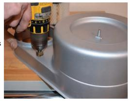
found a varia-bit to be the most effective tool for making this larger hole. No provision is needed for a mass air flow (MAF) sensor, as our Holley management will tune on speed density (part of the reason we chose said management system).
