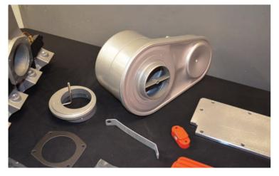
With the throttle body squared away, we move along to the icing on the cake: LS Classic's original style air cleaner. No hokey open element air filters here, we wanted this baby to look as original as possible, and they've got just the trick. Note the aluminum adapter with the stud to mate this original intake to our LS3's throttle body.
