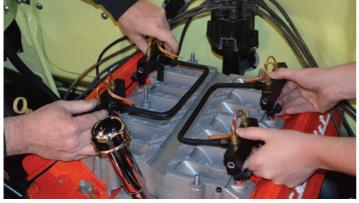
Before you bolt the upper plenum on, you'll reinstall the fuel rails/injectors. Leave them loose, as it'll help with getting the hoses lined up when setting the upper plenum on.
