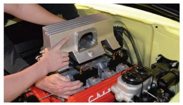
Setting the plenum on can be a two man job, with two hoses and four injector rails to manage. Having a buddy handy will make quick work of lining everything up.
