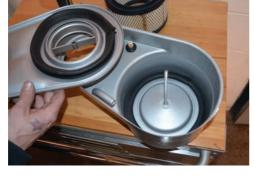
With our housing completely squared away, the provided air filter adapter can be mounted. This piece locks on to the throttle body via a hex set screw.
