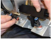
Set the injectors into the manifold first, then install the rail on the top side. A thin coating of petroleum jelly on the injector o-rings will help them install without pinching/
