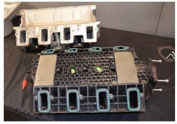
Put a ring on it! With your injectors done, we'll move to the bottom. LS intakes utilize an o-ring to seal the intake to the head as opposed to the paper gaskets a standard small or big block would. Nice thing is, they're completely reusable, and provide an ultimate seal.
