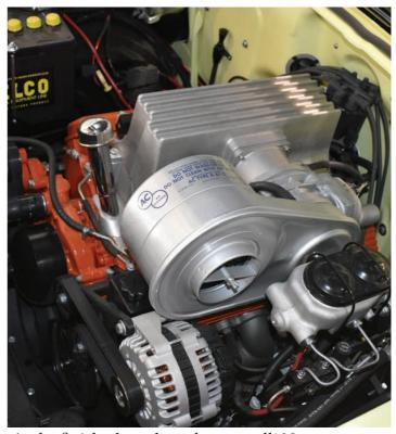
And a finished product shot as well! Note our use of LS Classic's accessory drive setup as well, a neat piece that minimizes the front drive, and utilizes a built-in power steering pump reservoir.
