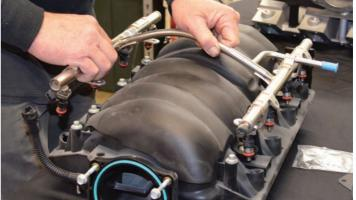
Go ahead and remove the throttle body and the fuel rails/injectors. Unless you're doing significant engine upgrades at the time of the intake manifold, the stock injectors and throttle body supplied with your engine, such as our 376/480 crate motor, will be just fine.
