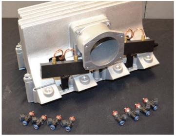
Injectors are not location specific, but simply need to be installed nozzle (in this case, red o-ring side) down.
