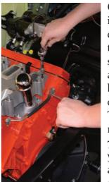
Once the o-rings are installed, the lower intake can be bolted into place. Do take note, these are VERY small bolts, going into an aluminum head. Care must be used to not break them off and/or strip the threads. These get tightened just north of hand tight, between 7-10ftlbs. Remember, all you're doing is compressing an o-ring, not squeezing down a paper gasket.
