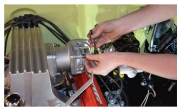
....then install the throttle body itself. Again, we chose to use the factory drive-by-wire throttle body. Our Terminator X-Max computer is made specifically for DBW, so the connection is a true plug-and-play. Combine that with a Woody's Hot Rodz LS pedal bracket (P/N WHR-30401) to mount the pedal provided in our Connect and Cruise package, and this installation only gets easier!
