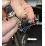
With the rails removed, you can remove the retainer clips that hold your injectors in, and remove them from the rail itself.
