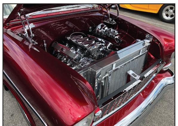
Vintage Air, and sheetmetal aluminum intake manifolds from Holley's Sniper line make quick work of taking the LS from a mundane looking piece intended to be hidden, to a gem that can stand front and center without faltering.
