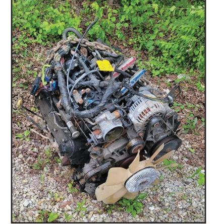
the cards before installation, I personally prefer to stay away from engines equipped with GM's "displacement on demand" or "DOD" setups. These setups can be failure prone in the lifter department if intending to use in stock configuration. Outside of that, you'd treat the buying and inspection process the same as you'd treat a small block Chevy. Lower miles, the better, well maintained the better. And the better you start, the better you end up.
